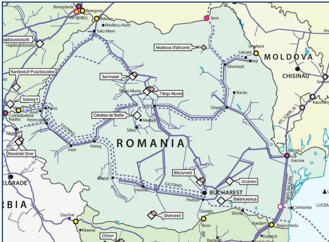
Gas Transmission Infrastructure in Romania Source: ENTSOG
